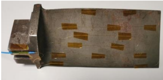
FIG. 7: Small compressor blade instrumented with a FBG sensor in the frame of SDS POC
