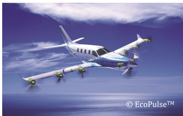
FIG. 2: EcoPulse hybrid-electric demonstrator developed by Daher, Safran and Airbus with the support of France's CORAC
